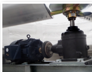
Standard: Gear Drive System
