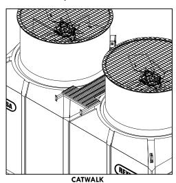
Corrosion-resistant FRP grating, supported by stainless/galvanized steel structure.
