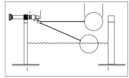
Figure B-1: Float valve installation
