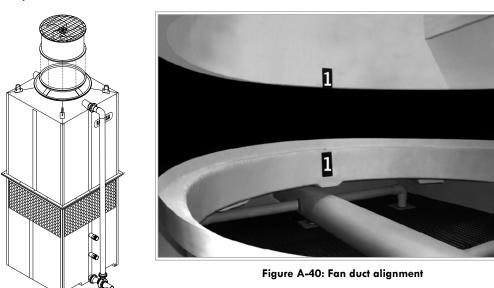
Figure A-39: Fan duct installation in a fan adaptor
