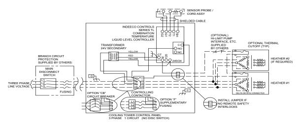
Figure A-57: Basin heater control panel diagram
