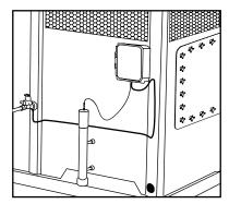
Figure A-58: Electrical Water level control system
