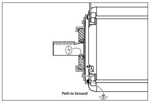
Figure A-60: Motor Shaft Grounding Ring
