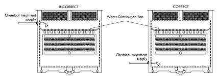
Figure C-10: Chemical treatment connection installation.
