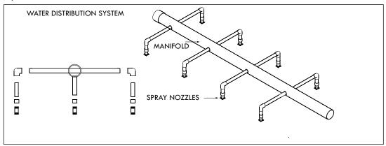
Figure C-9: Water distribution system schematic drawing
