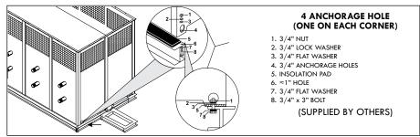
Figure A- 29: Typical anchorage for HFC-F models
