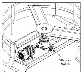
Figure A-49: Vibration Switch recommended location for HFC-F models.
