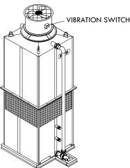
Figure A-44: Vibration switch recommended location
