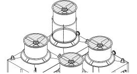
Figure A-41: Fan duct installation in a fan adaptor for a four fan tower
