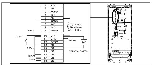
Figure C-6: Recommended Connection Diagram for ABB ACH550-UH.
