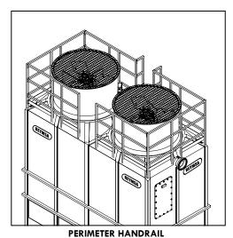
Stainless/galvanized steel railing OSHA construction, including toe guard.
