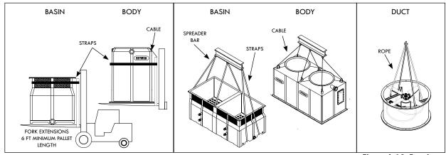
Figure A-10: Two fan tower fork lifting
