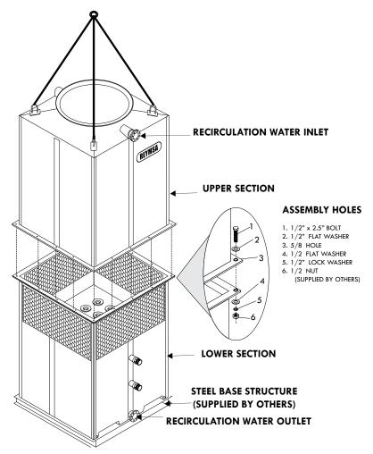
Figure A-7: Upper and lower parts installation
