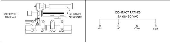
Figure A-45: Internal switches
