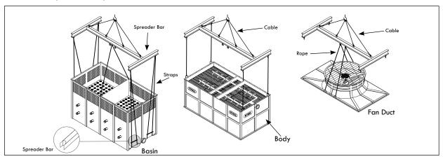
Figure A- 28: Crane lifting for HFC-F models
