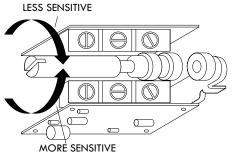
Figure A-48: Sensitivity adjustment
