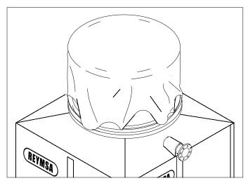
Figure C-12: Fan discharge covering
