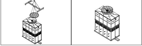
Figure A-32: Screen mersh assembly for HFC-F models
