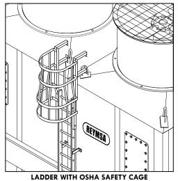
OSHA ladder and Cage with supports, stainless steel or galvanized steel.
