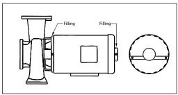
Figure D-1: Lubrication Points.
