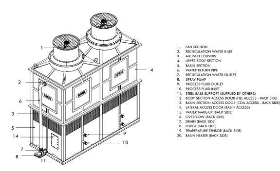
Figure A-65: Pipe connections for a double fan tower
