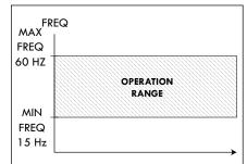
Figure C-1: VFD operation range for induction motors
