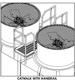
Corrosion-resistant FRP grating, supported by stainless/galvanized steel structure, with safeguard handrails on each end.
