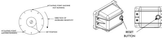
Figure A-52: Sensitivity adjustment
