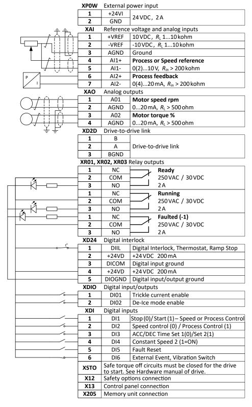
Figure C-7: Recommended Connection Diagram for ABB ACS880 Drive.
