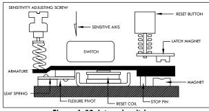
Figure A-50: Internal switches
