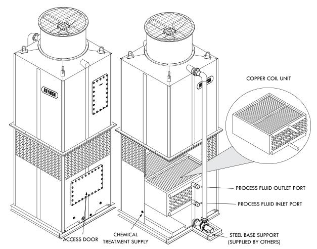
Figure A-34: Copper coil unit
