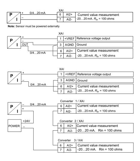
Figure C-8: Sensor connection examples for ABB ACS880 Drive.
