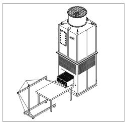
Figure D-3: Copper coil unit pulled out for maintenance purpose when tower is on the roof.
