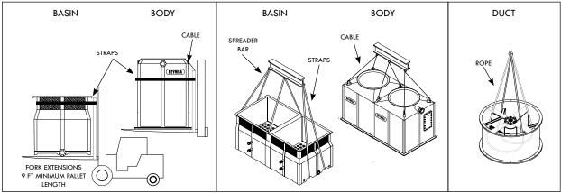
Figure A-18: Double fan tower fork lifting
