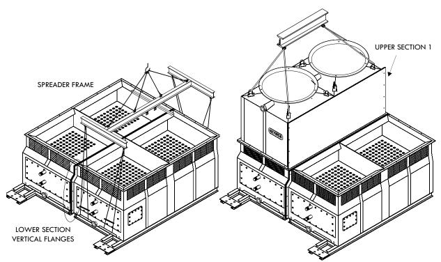
Figure A-23: Lower section installation for four fan tower
