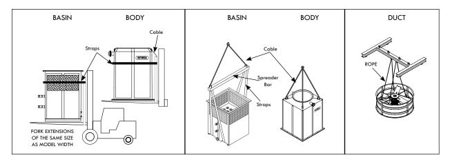
Figure A-3: Single fan tower fork lifting
