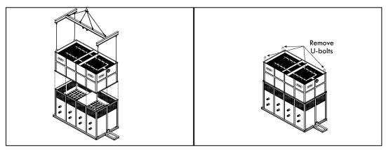
Figure A-30: Upper Body Section INSTALLATION for HFC-F models
